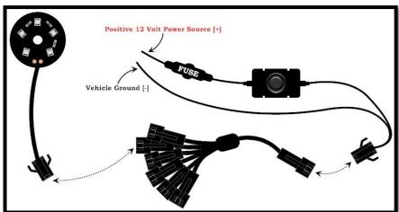
3. Begin by first laying out the pod lights similar to the way they will be installed. Make sure that the wires will be able to be routed in such a way that they will not be pinched, cut or exposed to heat. Also, keep the pod lights and wires away from all moving parts that may come in contact with any part of the kit. IF A POWER WIRE IS PINCHED, IT WILL CAUSE THE KIT TO MALFUNCTION AND WILL VOID THE WARRANTY DUE TO PHYSICAL DAMAGE.
